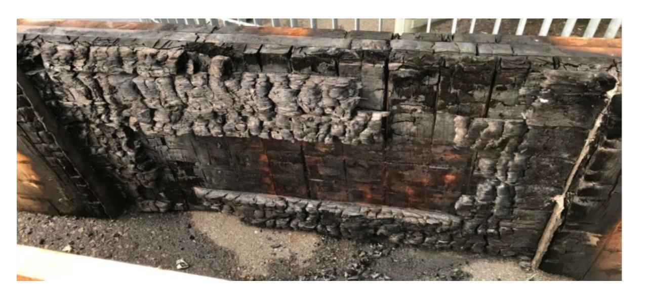
Test 1-6 (One Wall & Ceiling Exposed, Narrow Opening)
